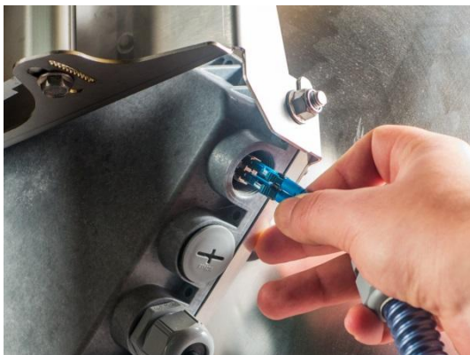
5 Connect LC connector to SFP module.
